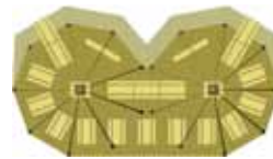
Duo, semi-raised, 90–120 seated 21 m x 11 m. With fireplaces and bar counters; relatively spacious.
